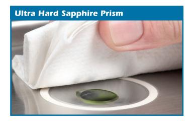
Some manufacturers use glass or YAG ( Yttrium-Aluminum-Garnet.) prisms. These prisms are softer than sapphire and have slower temperature transfer coefficients.
