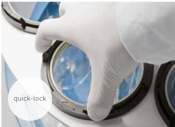
→ Auto-centering vessels with quick-lock system
