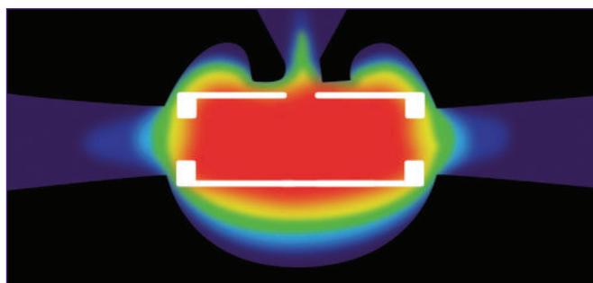
Transverse heating guarantees uniform temperature distribution in the graphite tube, even allowing the accurate analysis of refractory elements such as vanadium or molybdenum.
