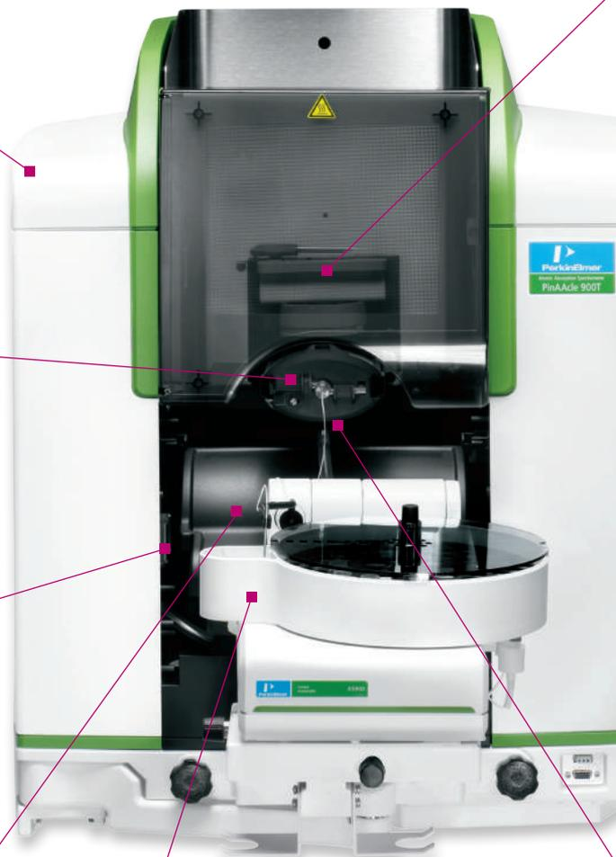
**Unique stacked flame/furnace design**—Requires only a single vent for all analytical techniques, simplifying installation and minimizing costs.
