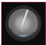
**TubeView color furnace camera**—Simplifies autosampler tip alignment and sample dispensing. Can also be used to monitor drying and pyrolysis during analysis for simpler method development.
