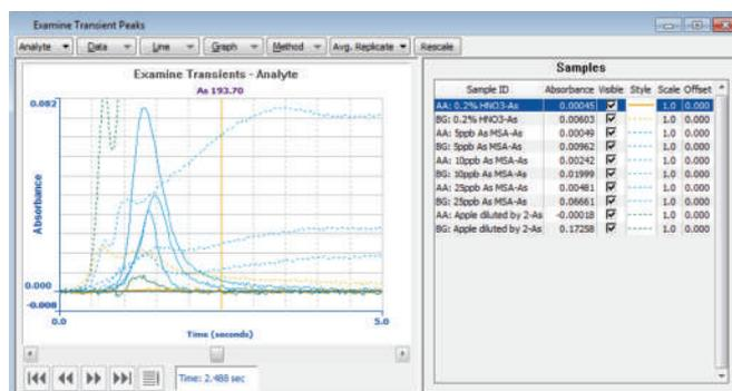
**Examine Transient Peaks Window** allows you to view the effects of changing various analytical parameters for accelerated method development.
