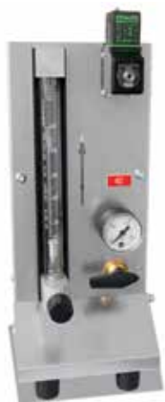
Gas supply system for non-flammable protective or reactive gas with shutoff valve and flow meter with regulator valve, piped and ready to connect
