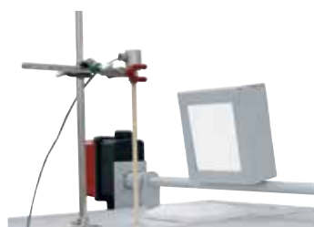
Exhaust air flap and charge thermocouple including a stand as additional equipment
