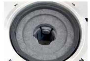
Graphite heating module
