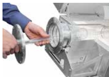
Gas tight closing plug for tubes made of quartz glass closed at one side
