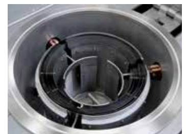
Cylindrical retort with tungsten heating
