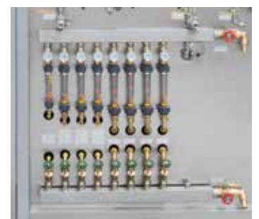
Cooling water distribution
