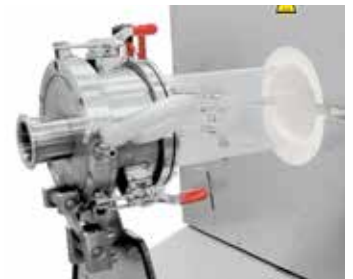
Quartz glass and flanges for protective gas operation as optional equipment
