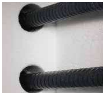
Furnace chamber with high-quality fiber materials and SiC heating rods on both sides of the furnace
