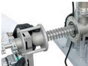
Screw-conveyor with adjustable speed
