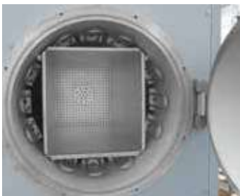
Inside heating in retort furnaces NRA ../06
