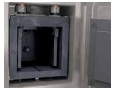
Graphite heating chamber
