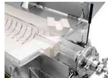
Adapters for alternative operation with working tube or process reactor
