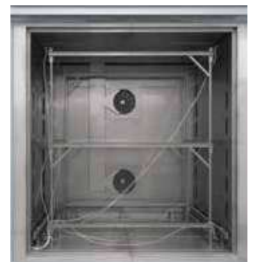
Pluggable frame for measurement for forced convection chamber furnace N 7920/45 HAS
