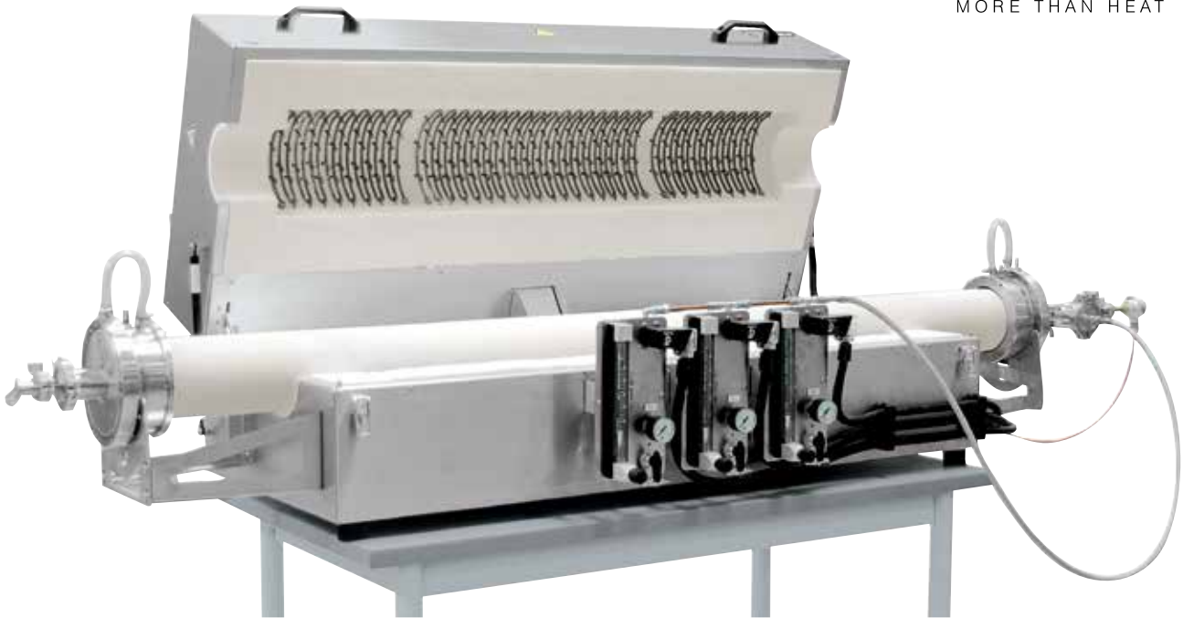
Tube furnace RS 120/1000/13S with gas tight tube, heating elements embedded in fiber module, charge control and check valve at gas outlet
