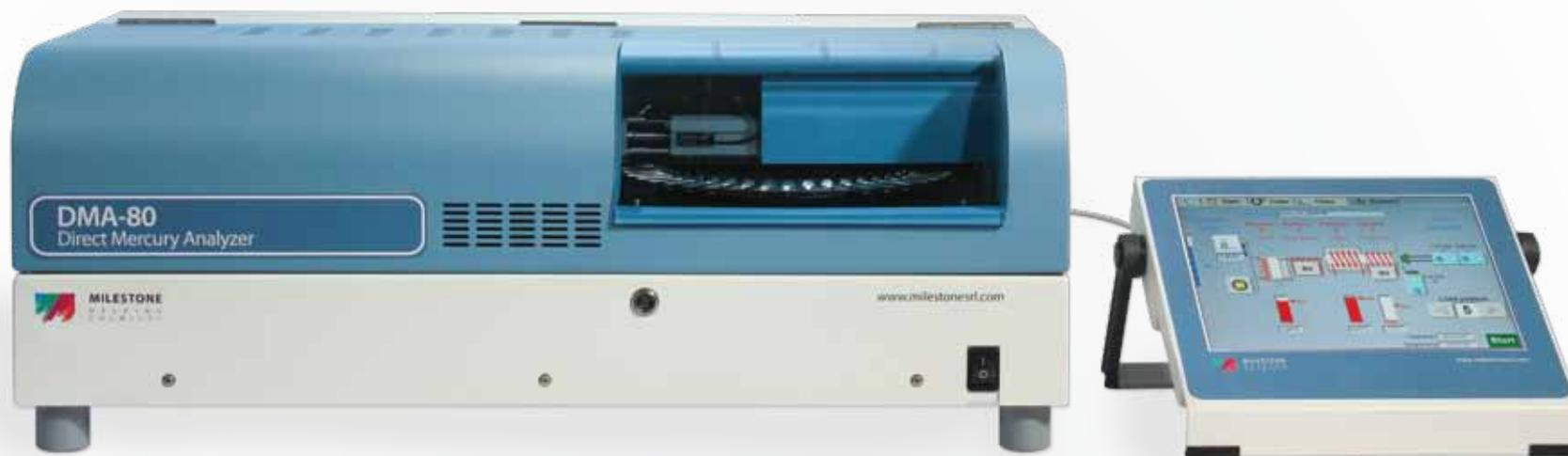
The Milestone DMA-80 is a direct mercury analyzer of solid, liquid, and gas samples. Analysis time is 5 minutes only and no sample preparation is required.
